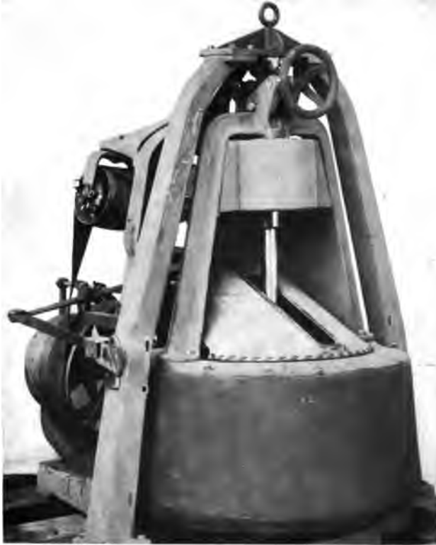
Fig. 1. Centrifugal Extractor with Cover.
